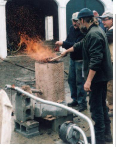
With the air blower on, the furnace roars into action. Here, Darrell Markewitz demonstrates how to smooth out the top of the ore-charcoal charge.
