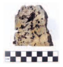
Sliced open, the iron in our bloom is easy to see, as are the air holes that a blacksmith will have to hammer closed.
