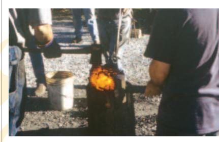
We carry the bloom to a hollowed log and split the bloom using an axe pounded by sledgehammers. To preserve its temper, the axe must be quenched frequently while it splits the still-hot bloom.
